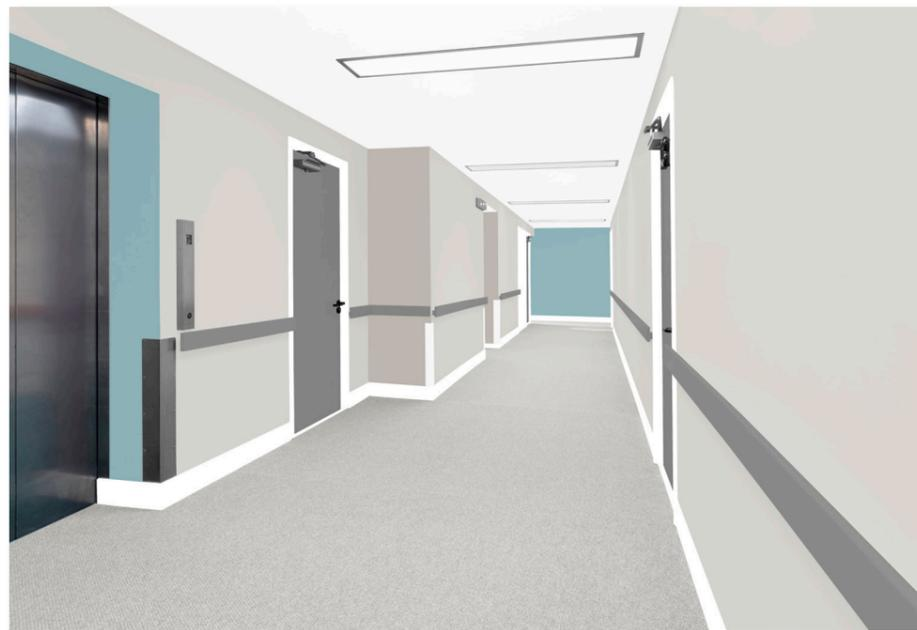
1. Within public spaces, all critical surfaces (walls, floors, doors and handrails) should be defined and have contrast between them. The recommendation is a minimum of 30 points of Light Reflectance Value (LRV).
